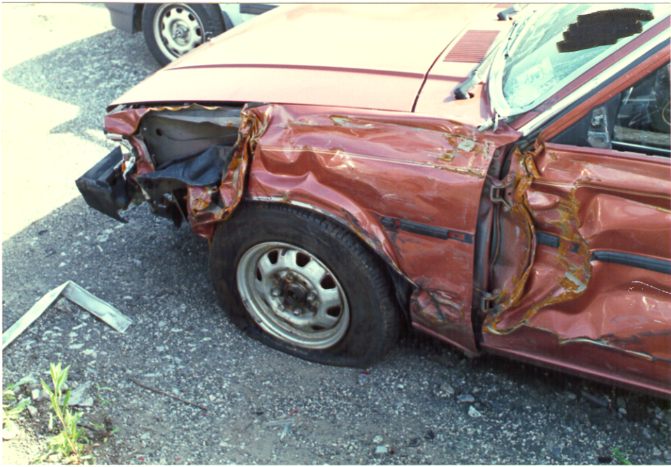
Rearward Displacement Of The Leading Edge Of The Left Front Fender and Door.
